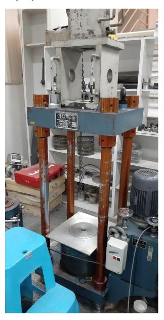
Facility Uniaxial & Triaxial Test Jack (Semi-Automatic)
