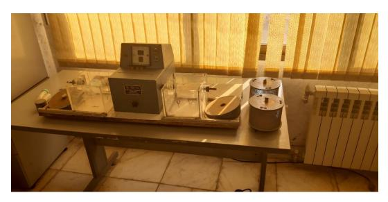
Facility Point Load Test Apparatus
