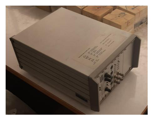
Facility Ultrasonic Wave Speed Measuring Apparatus
