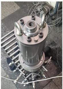
Facility Hook Triaxial Cell Test
