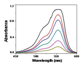
Fig. 8.3 Photodegradation of RhB collected at intervals of 15 min over an exposure period of 75 min with nano  $Bi_2O_3$
