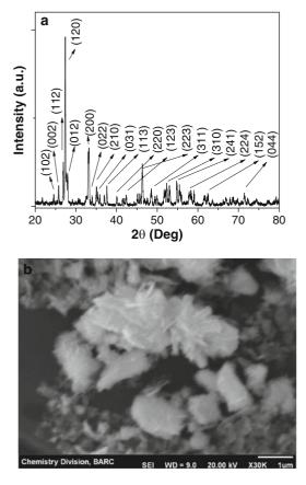
Fig. 8.2 (a) XRD pattern and (b) SEM image of sonochemically synthesized  $\rm Bi_2O_3$
