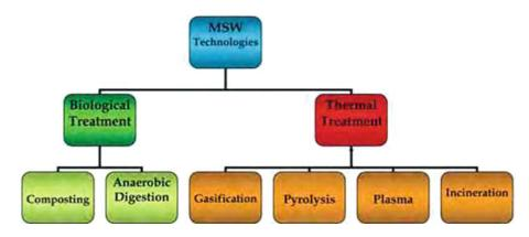
Fig. 1.2 Different biological and thermal methods for solid waste management
